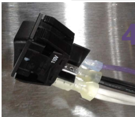
Convection fan switch as wired from factory (note purple wire may also be blue)
